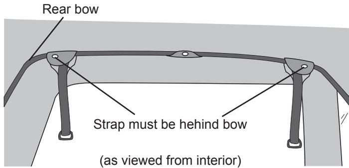
**Step Five:** Make sure that the straps sewn into the rear of the top are behind the rear bow.
