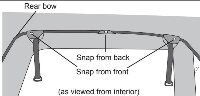
**Step Seven:** Snap the top to the rear bow. The center snap flap will wrap around the bow from behind and the two outer snap flaps will wrap around the bow from the front.
