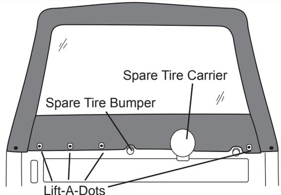
**Step Nine:** Fasten the bottom of the Rear Curtain to the Lift-A-Dots on the rear of the vehicle.
