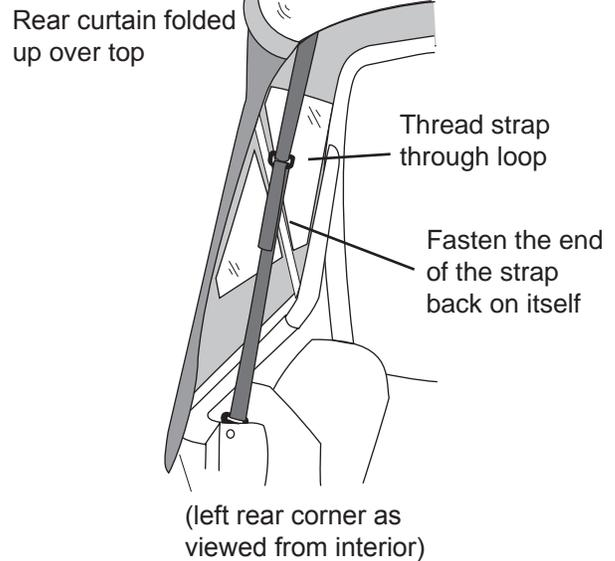
**Step Six:** Thread the Tension Straps through the loop on the strap sewn into the rear of the top. Pull the strap tight and secure it in place with the hook & loop sewn to the strap. **NOTE:** Pull the strap down tight but do not use excessive force, it is not designed to pull the bow assembly downward.
